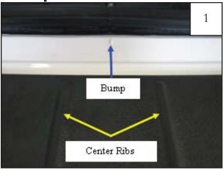
Open rear door of vehicle. WITHOUT peeling liner from tape pads, align part on bumper, centering the bump on rear door sill BETWEEN two center ribs of the bumper guard
