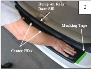
Apply a piece of masking tape along both edges of part for ease of placement during installation.
