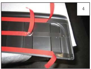
Peel the red plastic liner from the tape strips located on the inside of the bumper protector. NOTE: Make sure tabs are folded toward the outside of the part and that the middle tape liner is in front of rear liner.
