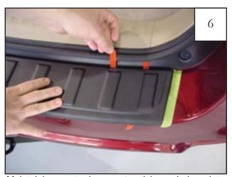
Maintaining part placement, stick peeled end to bumper and begin pulling center tab. Continue pulling center tab while applying pressure. Repeat process for liner the front of the vehicle, and the liner towards the back of the vehicle.
