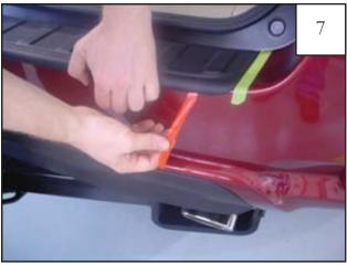
When peeling liner along front edge of part, run edge trim tool along under part in front of liner to create a small gap for ease of liner removal.
