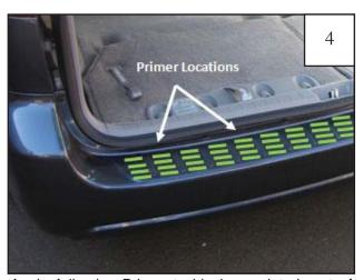
Apply Adhesive Primer to black unpainted part of bumper, between raised surfaces.
