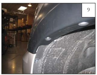
Install a supplied Retainer (RV1-P006) through forward hole in flare.
