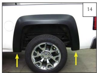
Reinstall the lower 2 factory fasteners removed in Step 5 using a 10mm deep socket and wrench.
