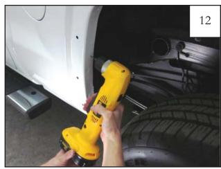
Using a 3/32" drill bit, drill pilot holes through sheet metal at the marks made in Step 11.
