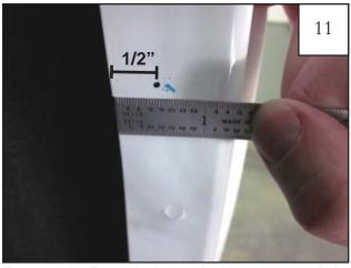
Remove the flare. At the marked locations made in Step 9, measure inward 1/2" from the inside edge of the fender and make a new mark. This is the mark to be drilled.
