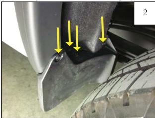
Using a T-15 Torx bit, remove the 4 factory screws from the plastic wheel well piece and remove.
