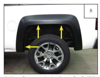
Hold rear flare up to wheel well to confirm fit. While holding flare on vehicle, install supplied screws (SW1-0056) into the 2 upper and 1 lower factory hole locations. Do not fully tighten at this time.
