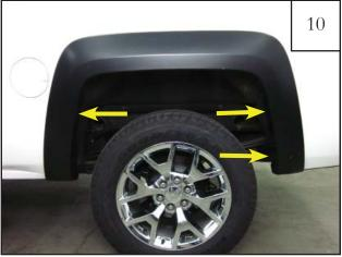
Hole locations to be marked for drilling.
