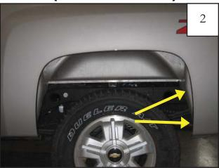
Remove two factory screws with a #2 stubby screwdriver.
