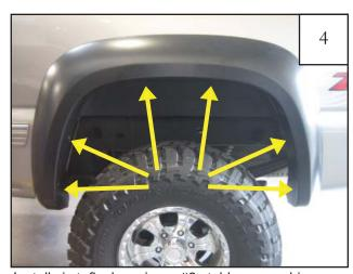
Install six tuflocks using a #2 stubby screwdriver.
