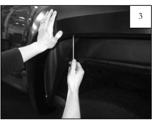
Align flare on vehicle and start a supplied screw (SW1-0058) through the two uppermost holes in the flare and into each clip installed in Step 2. **DO NOT FULLY TIGHTEN SCREWS AS THEY WILL BE UNINSTALLED**
