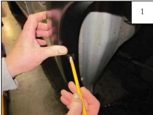
Hold flare in position on fender. Aligning top two holes in flare with factory holes in sheet metal, use the remaining four holes in flare as a guide to mark sheet metal with a grease pencil.
