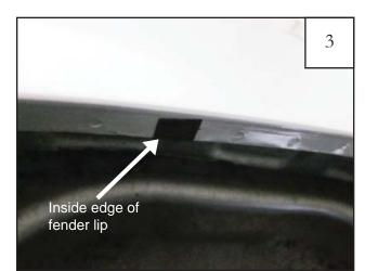
Center a supplied Tab (MT1-0002) over all four marks made in Step 1 and the two factory holes, aligning edge of Tab with inside edge of fender lip (Tab may extend over outside of fender).
