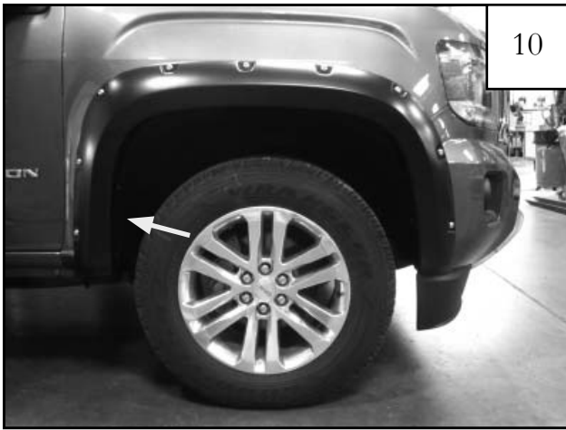
Holding the flare into position on vehicle, use a grease pencil or sharpie to mark sheet metal using the upper rear hole location as a guide.
