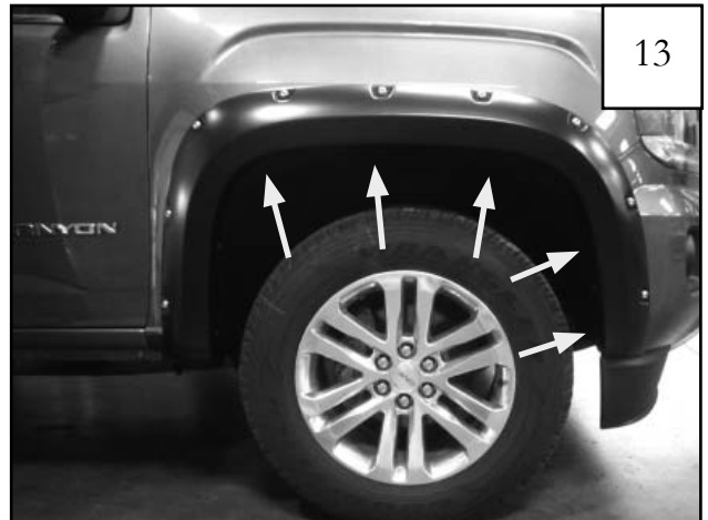
Holding flare in position, start five supplied screws (SW1-0056) into the top three and front two holes. Do not fully tighten.
