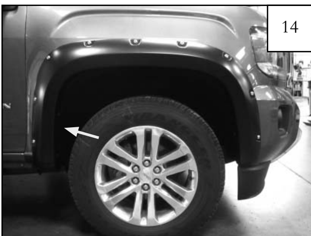
Using an awl, align clip with mounting hole and start one supplied screw (SW1-0056). Do not tighten.
