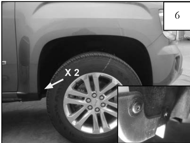
Using a T-15 torx bit, remove two factory fasteners from mud guard. Discard factory fasteners only..
