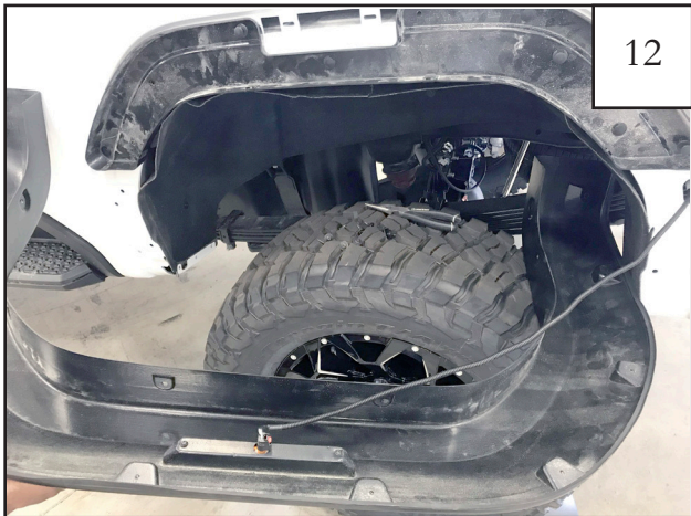
Connect electrical wire for light and run inside flare.
