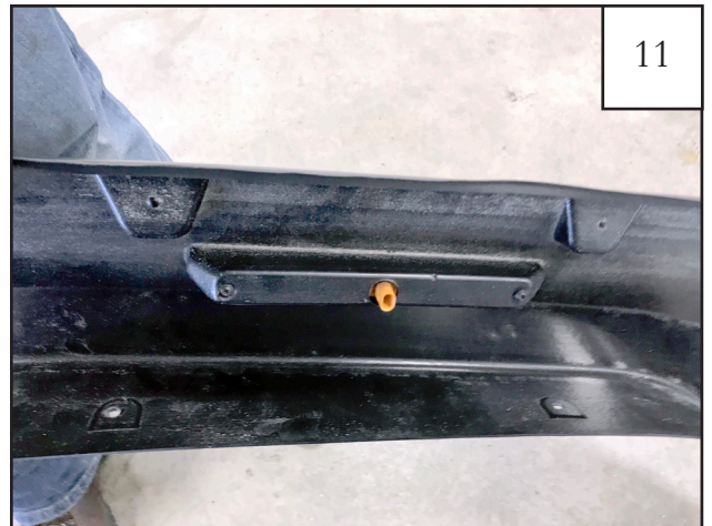
Install light in new flare using (2) torx screws removed in Step 5 .
