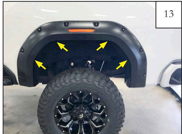
Use (4) Truss Screws (SW1-0058) to install flare on to U-Clips (CL1-0022) on inner bracket
