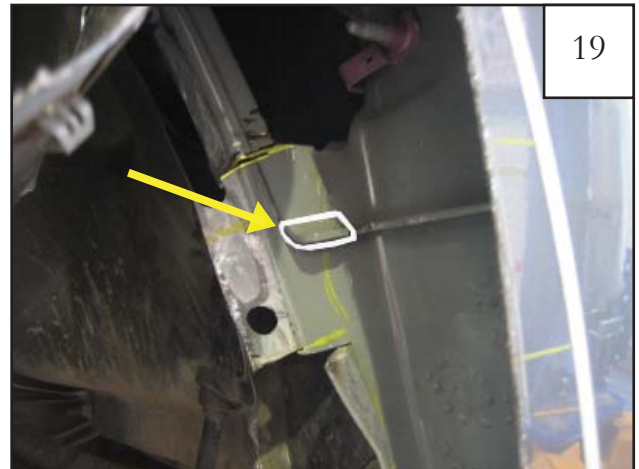
19 Cut off outlined tab to make bend in the next step easier.
