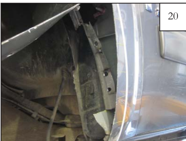
20 Bend inner support over and use a hammer to flatten against wall inside fender.
