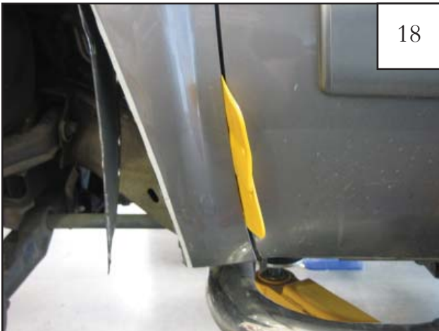
18 To prevent paint damage, insert plastic spacer between fender and door. This will keep the fender from hitting the door edge while pounding back sheet metal in the next few steps.
