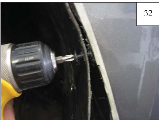
Starting with the top location, fasten inner fender metal to bent tabs of outer fender with Screw (SW1-0056)s through holes drilled in last step (3 locations).
