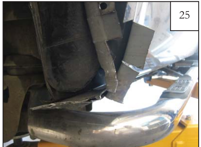
Bend remaining metal back even with other tabs.
