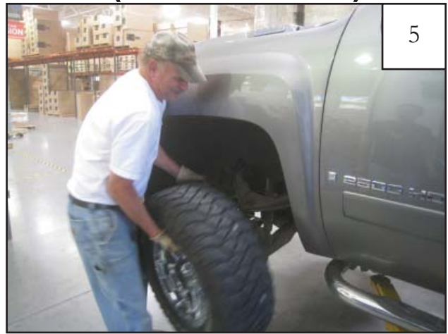
Support vehicle and remove tire.
