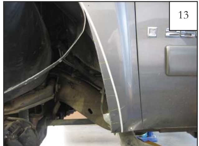
Bend inner fender metal away from fender.
