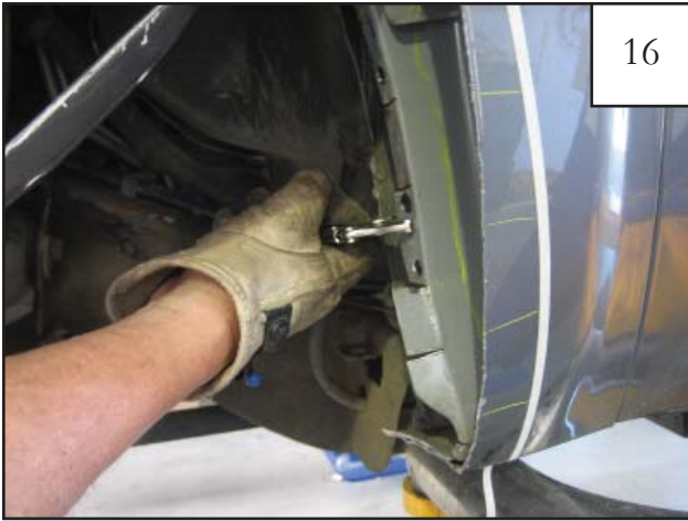
16 Bend lip straight with pliers between cuts made in previous step.
