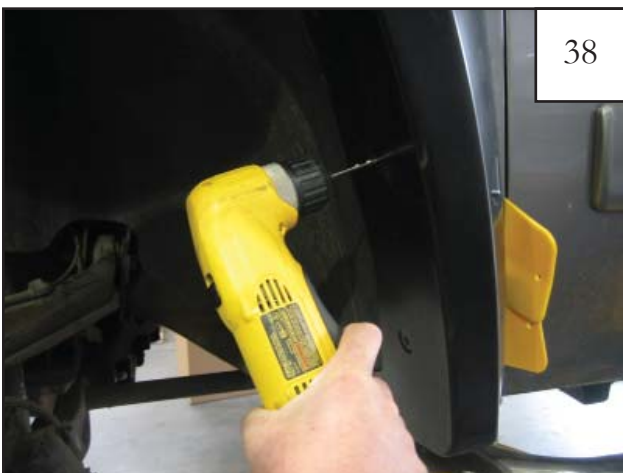
At two locations in the rearward side of the flare, drill through hole in flare and into sheet metal of vehicle.
