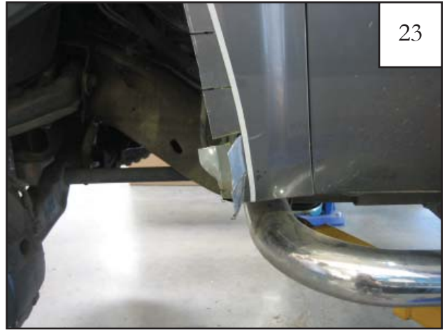
Bend lowest two metal tabs outward.
