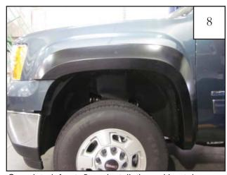
Completed front flare installation without bumper piece.
