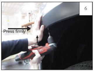
Check that flare is positioned correctly around wheel well. If not, adjust before tightening screws. Then, making sure bumper piece and flare seams are still aligned with factory seams, *firmly* press the flare up and toward the vehicle while tightening all screws.
