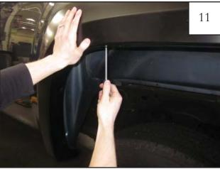
Align flare on vehicle and start a supplied screw (SW1-0058) through the two uppermost holes in the flare and into each clip installed in Step 10. **DO NOT FULLY TIGHTEN SCREWS AS THEY WILL BE UNINSTALLED**
