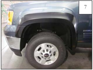
**OPTIONAL BUMPER PIECE:** Completed front flare installation.
