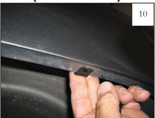
Center a supplied Clip (CL1-0022) over the two holes in Step 9. Clips may need to be adjusted to align with holes in flare. *Note: The raised collar on the Clip should face upward into the interior of the fender.*
