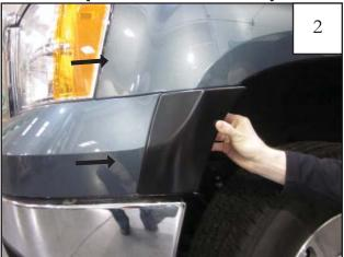
**OPTIONAL BUMPER PIECE:** This vehicle comes with different bumper sizes. If installing the optional bumper piece, verify which piece to use by holding it up to the bumper and making sure it lines up with factory edges and hole locations. After identifying bumper piece, apply edge trim along outer surface.
