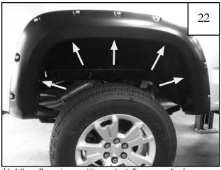
Holding flare in position, start five supplied screws (SW1-0056) starting through the top center hole working outward. Use awl to align clip with mounting hole.
