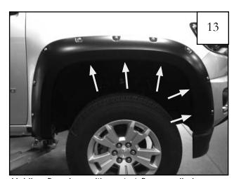
Holding flare in position, start five supplied screws (SW1-0056) into the top three and front two holes. Do not fully tighten.
