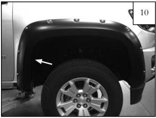
Holding the flare into position on vehicle, use a grease pencil or sharple to mark sheet metal using the upper rear hole location as a guide.
