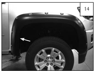
Using an awl, align clip with mounting hole and start one supplied screw (SW1-0056). Do not tighten.
