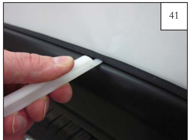
41 Using flat end of supplied Edge Trim Tool (ET1-0002), seat edge trim against flare by inserting straight end between edge trim and flare at one end. Next, slide around entire edge to the other end.
