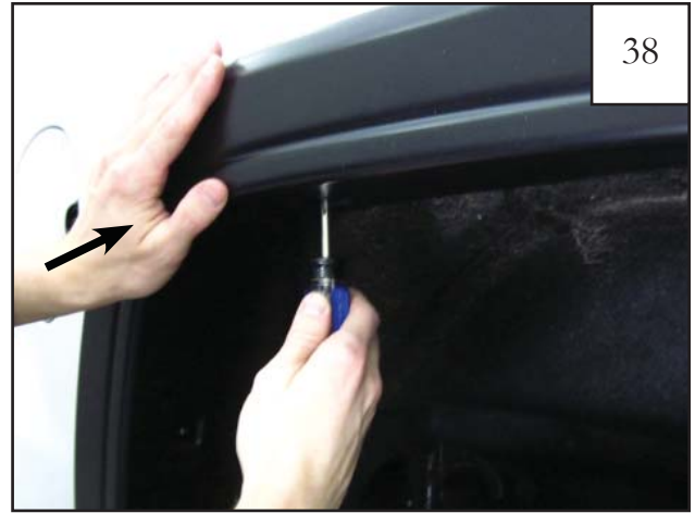
38 Press flare towards vehicle and fully tighten all remaining fasteners.
