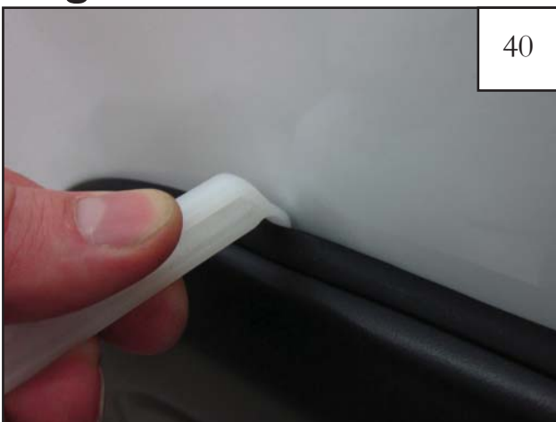
40 Using supplied Edge Trim Tool (ET1-0002), seat edge trim against vehicle by hooking curved end under edge trim at one end of flare. Next, slide around outer edge of flare to the other end.
