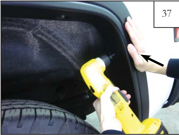
37 Install self-tapping screws (SW1-0066) into pilot holes drilled in step 36 (3 places). Press flare firmly towards the vehicle while fully tightening.
