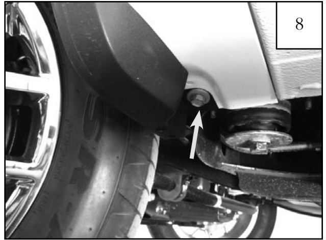
Remove fastener from rear underside of factory wheel arch molding using a 1/2" socket and wrench. Save for reinstallation.
