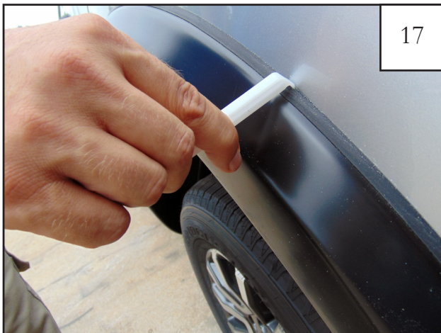
17 Using supplied Edge Trim Tool (ET1-0002), seat edge trim against vehicle by hooking curved end under edge trim at one end of flare. Next, slide around outer edge of flare to the other end.
