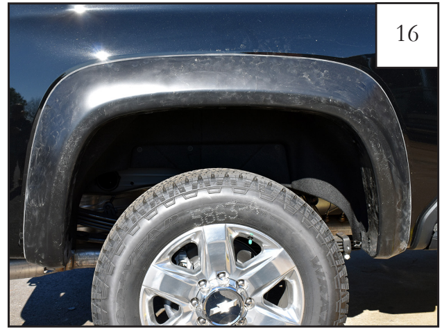
16 Fully tighten all fasteners, then replace the rear wheel as instructed in your user's manual. Rear flare installation is complete. Repeat procedure for opposite side.
