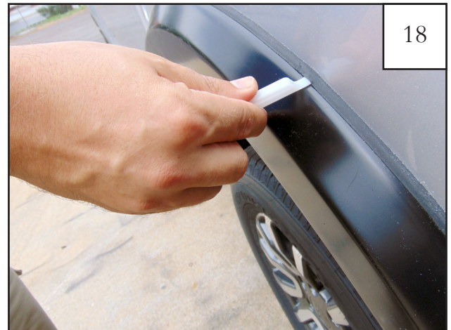
18 Using flat end of supplied Edge Trim Tool (ET1-0002), seat edge trim against flare by inserting straight end between edge trim and flare at one end. Next, slide around entire edge to the other end.
