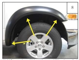
Hold flare to the vehicle and start additional supplied screws with a Phillips Head Screwdriver through the factory holes. *Do not tighten*.
