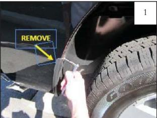
**2012 Models Only (Optional):** If you encounter a fit problem, remove inner piece at bottom rear <u>and</u> front of wheel well.
