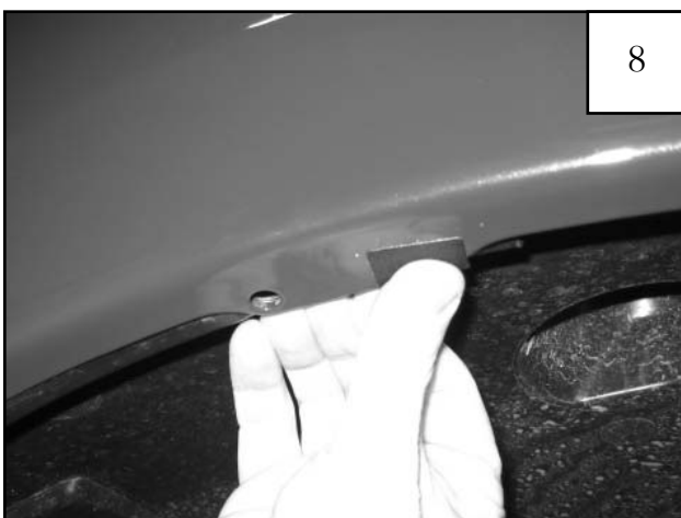
Install plastic tab over existing factory hole.
