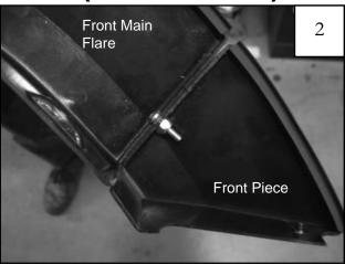
Bolt front main flare and front pieces together with supplied screw (SW1-0003) and supplied nut (NU1-0004). Use a 3/8" wrench to hold nut in place.
