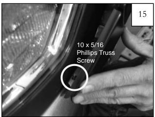
When fitting flare on vehicle, first position front piece. The Truss Tap Screw (SW1-0050) hooks behind where folded 1"x1.5" Black Tab was installed in step 6.
