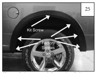
Kit supplied screw and factory installed screw locations. See Steps 26 & 27.
