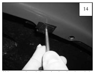
Using an awl or similar pointed tool, poke a hole through 1"x1.5" Black Tab using the clip hole as a guide.
