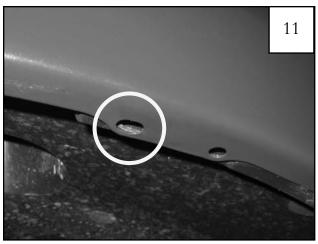
At location indicated in step 10, there is a lip with two factory holes. One hole is a circle and one is an oval. The 1"x1.5" Black Tab (MT1-0014) and clip (CL1-0022) will be installed over the oval. The oval is the hole more toward the front of the vehicle.
