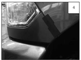
Install two 1"x1.5" Black Tabs (MT1-0014) over seam between main vehicle body and headlight mounting.
