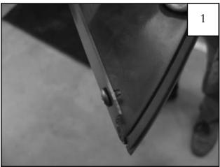
Using dimple in front piece as a guide, drill a 1/8" hole and install supplied screw (SW1-0050) through the drilled hole.
