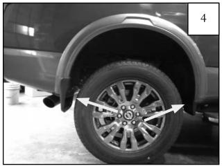
If Factory Mudflaps are installed, use a #2 Phillips Screwdriver to remove them.
