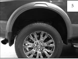
If Factory Flares are installed, use a #2 Phillips Screwdriver to remove them. If no Factory Flare is installed, go to Step 17.
