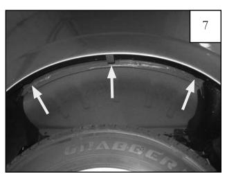
Install a foam tab (MT1-0034) over 3 top center metal tabs in the wheel well
