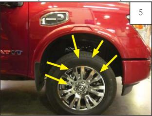
Using a #2 Phillips Screwdriver, remove factory flares if installed.
