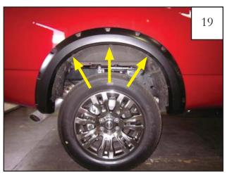
Position flare on rear fender and install 3 supplied screws (SW1-0058) through flare and into the clip holes.
