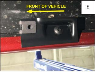
Use factory screw to install inner bracket in wheel well where shown.
