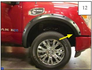
Install a supplied push retainer (RV1-P001) into the hole drilled in the previous step.
