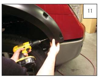
Push in on the front of the flare. Using a drill with a 1/4" bit, use the hole in the flare as a guide and drill a hole into the wheel well.
