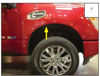
Using a #2 Phillips Screwdriver, remove factory screw from wheel well.
