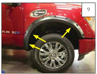
Position flare on fender. Line up holes in flare with the factory holes and start the two 3 supplied screws (SW1-0049) where indicated in picture. *Do not fully tighten screws*.
