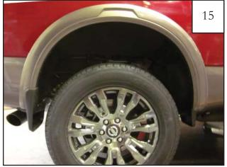
If Factory Flares are installed, use a #2 Phillips Screwdriver to remove them. If no Factory Flare is installed, go to Step 17.
