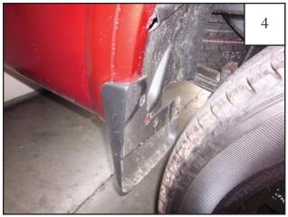
Using a #2 Phillips Screwdriver, remove factory mud flaps if installed,
