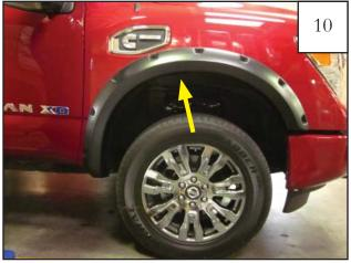
Install a supplied screw (SW1-0056) into the hole in the flare and into the bracket. Tighten all screws.
