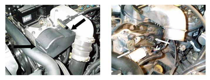
The plastic cover is held in place by 2 plastic Phillips head screws, only light pressure is required to remove them. Do not lose the screws or washers when you remove them. Remove the cable from the throttle linkage and support bracket.
