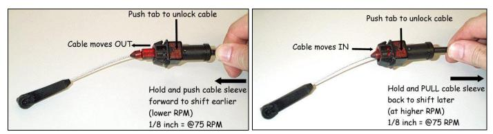
Adjusting the cable forward, towards the radiator, will make the transmission shift sooner.
