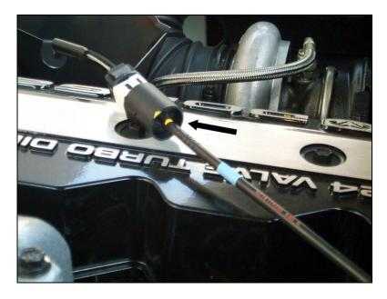
\*\*IMPORTANT: MARK THE CABLE at the original setting before any adjustments are made.
