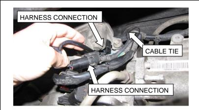
6. Remove lower dash panel and route switch harness from steering column area through grommet in firewall and connect into module harness.
