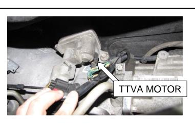
5. Cable tie wiring along transmission across to the frame rail and up the firewall.
