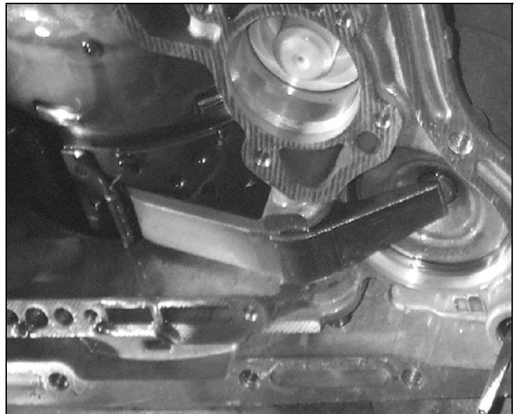
New BD band strut in place
