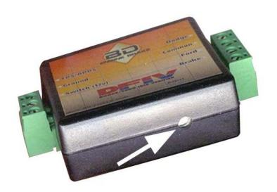
screw in the DFIV Module counterclockwise or clockwise until the test light JUST turns on.
