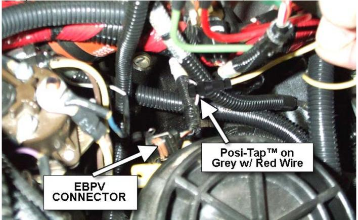
FORD 1999-2003 (7.3L) Locate the wire harness at the EBP Valve and peel back the insulation to allow access to the wires. Locate and attach a Posi-Tap<sup>TM</sup> to the Grey w/Red tracer wire.
