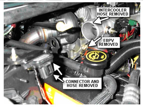
For ease of access and hook up, remove the connector from the EBP Valve and pull the wiring through and underneath to the front of the intake Y-plenum. This will allow access to install a Posi-Tap™ or Connector harness.
