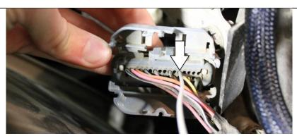
35. Crimp the supplied terminal onto the black wire from the LED. Install into position 20.
