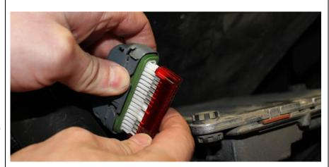
11. Remove the RED retainer on the vehicles transmission harness connector. Install the supplied BLUE retainer. Keep the removed RED key incase the module is ever removed.
