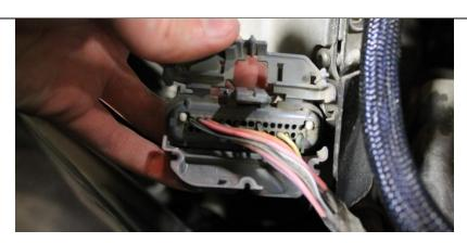
34. Insert the single wire from the tap shifter harness in position 12. Ensure wire is locked into the connector adequately by lightly tugging on the wire once installed.
