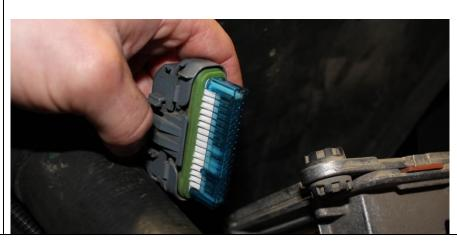
12. Connect the BD Tap Shifter wiring harness RED connector to the vehicles transmission control module.
