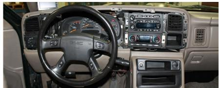
Remove the two 7mm screws from the bottom of the knee bolster and pull bolster outwards.
