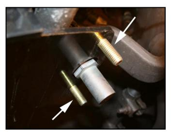
Install the bearing assembly over the sector shaft nut until the bearing block comes to rest on the support bracket (noting that the block may not be flat to the mount at this point).
