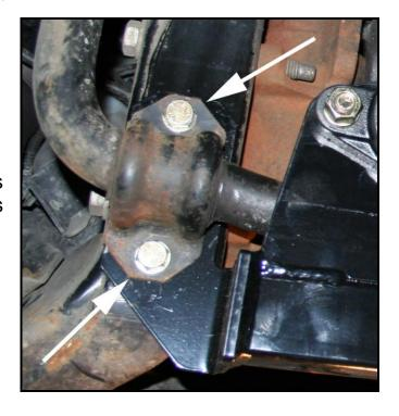
Ensure free movement (rotation) of the steering box sector shaft nut. If it is not free moving, then undo the sway bar bolts and readjust.
