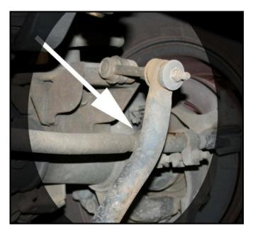
A **1-5/16**" **socket** will be required to remove the steering box sector shaft bolt with lock washer. Retain the lock washer for re-installation with the new nut.
