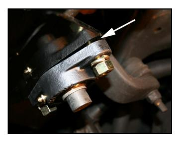
Tighten the four sway bar mounting bolts (17mm) to 40 lbs-ft. (as per Dodge's specification).
