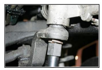
Slide the support bar into place, where the mounting feet are positioned in between the sway bar mounting and the frame.
