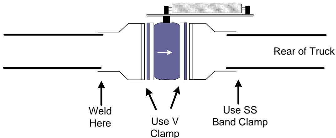
Temporarily mount the exhaust valve assembly on the adapter, with the supplied V clamp on the valve sliding. From here, cut off as much of the remaining exhaust needed to accommodate the valve and remaining adapter. Remove the exhaust valve assembly and clamp, or weld the rear adapter to the other section of exhaust pipe.
