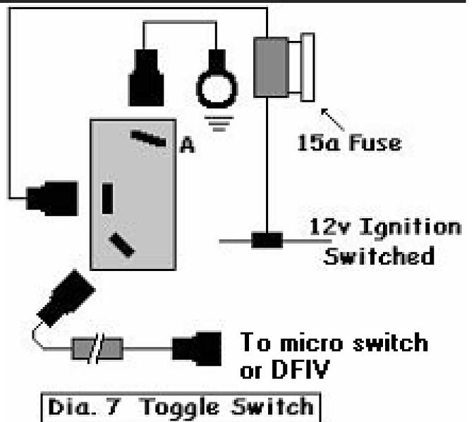
terminal on the micro switch to the exhaust brake control valve you mounted earlier. Route this wire away from any heat sources or moving parts.
