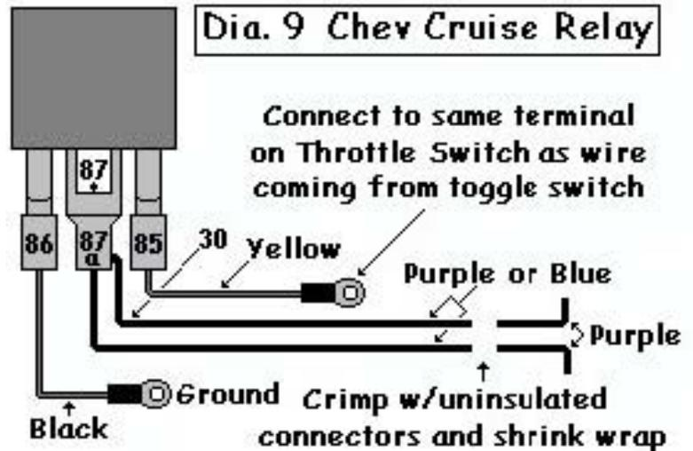
One of the purple wires leads up to another 8-pin connector just above it. You can verify the wire by tapping the wire with a test light and grounding the clip; with the ignition turned on the light should be illuminated, but no light when you press on the brake pedal. Cut this wire and connect both ends (see Diagram 9) to the purple (or blue) wires coming from the supplied relay using non-insulated butt connectors and shrink wrap.
