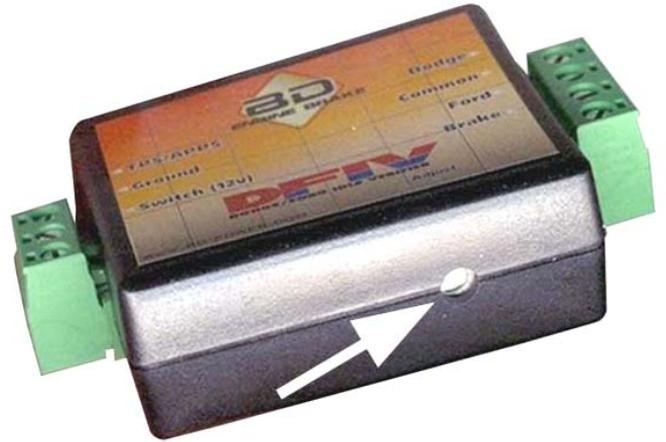
Connect one end of a test light to the "BRAKE" terminal of the DFIV module and the other end to a good ground. With the throttle at idle, start the engine and turn on brake switch. Then, using a small flat bladed screwdriver, turn the small adjusting screw in the DFIV Module counterclockwise or clockwise until the test light JUST turns on.
