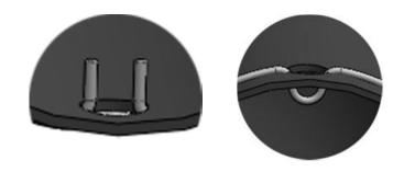
Now slip the small side of the boot over the bead ring and pipe assembly.
