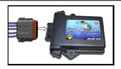
13. Locate the PAS valve solenoid connector. Then but connect the violet wires from the switch & solenoid to the violet wire from the module and heat shrink the connection.
