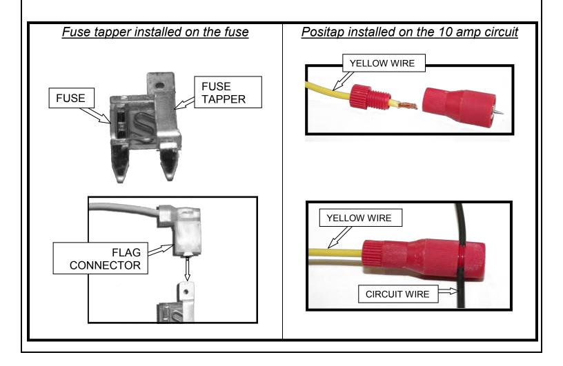
20. Double check all wiring connections and ensure wires are routed away from any heat sources and moving parts. Then install the loom with the supplied tee connector and clips for the loom ends and continue to the Setup, Testing and Verification with Over Speed Electronics section in this manual.
