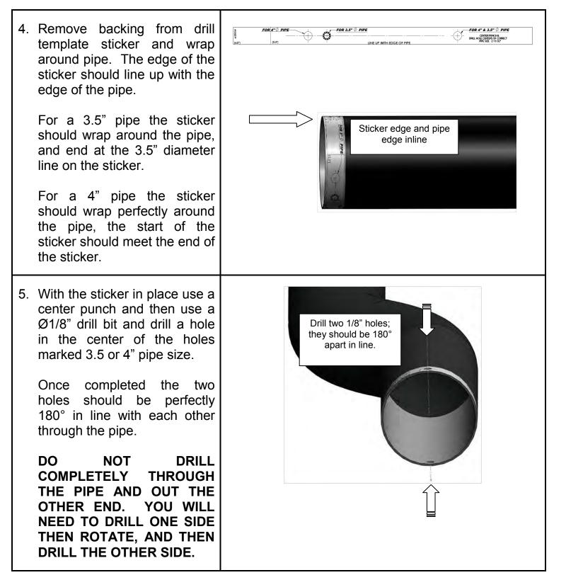
Once the pilot holes are drilled you will need to drill a Ø11/32" hole through the pilot holes.
