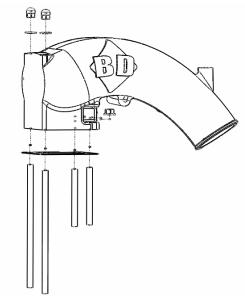
Reuse the factory dipstick tube mounting bolt to secure the dipstick to the intake.
