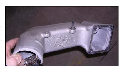
You will now need to scrape off any left-over gasket material that resides on the intake heater.
