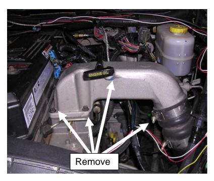
On the rear of the intake you will notice a wiring harness bolted to the intake. You will need to remove the nut and washer that secure the wiring harness to the intake.
