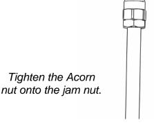
Note that the end with the shorter length of thread, should be inserted into the head.
