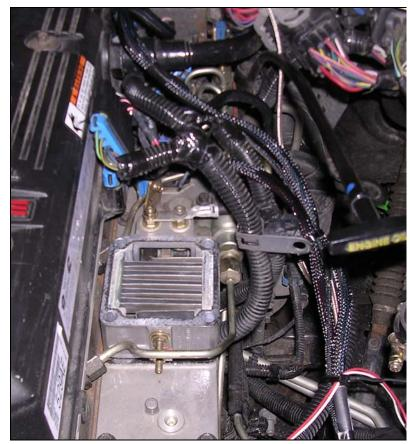
Place the new gasket (supplied) in place on top of the intake heater.
