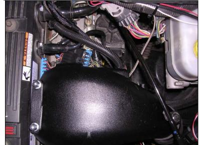
You can now reconnect the factory silicone boot and clamp. Be sure to clean the inside of the silicone boot with either an non oil based electrical contact cleaner or brake clean.
