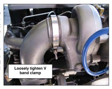
30. Install the *primary turbo* support bracket to the engine block with the supplied bolt (12mm x 1.75 x 25) and lock washer. Now tighten the bolts and V band clamp.
