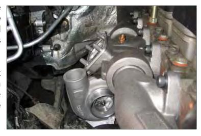
29. Using the supplied v-band clamp (clamp will be labeled 995L2-0406) tighten the secondary exhaust housing to the primary turbo-turbine adapter assembly.
