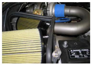
Note: The exhaust housings of the turbos may smoke slightly when new, as manufacturing residue on housing must burn off.
