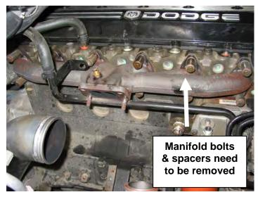
15. Reinstall the exhaust manifold in an <u>inverted manner</u> so the turbo flange faces upward. Use the provided manifold gaskets and the factory bolts, spacers and retainers and torque to 32 ft lbs with a 13mm socket.
