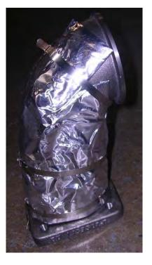
26. You can know bolt the flanged turbine adapter to the primary turbo. Use the four M10x1.25x30 FINE threaded bolts and washers to secure the two. At the same time mount the SS primary turbo support bracket to the assembly.
