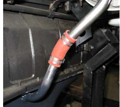
secondary turbo drain. This hose will attach to the factory drain adapter. Use the hose clamps to secure the connection. You will need to slide the oil drain adapter as far as possible away from the wastegate arm to prevent any contact. In some rare cases the wastegate arm may need to be bent.
