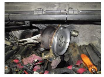
9. Clean the turbo shaft & lubricate it liberally with clean engine oil. Spin on the BD Compressor wheel (17mm), you should be able to spin it on by hand. If it does not go on freely chase the threads in the compressor wheel with a 1/4"NF tap. Torque the wheel to 85-115 INCH POUNDS. Make sure the wheel & shaft assembly spins freely after the wheel is installed.
