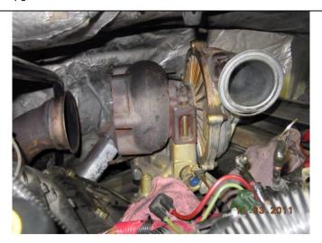
Remove the warm-up valve & it's housing from the back of the turbo by undoing the bolts (5/16" 12-point) & valve actuator rod. These bolts are often seized in place & can be difficult to remove.
