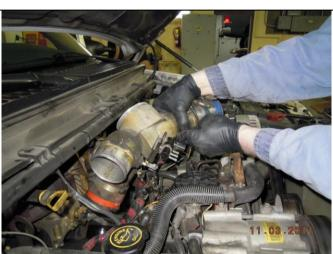
4. Remove the two nuts on the wastegate actuator (10mm). Use shop air to gently extend the actuator so that it extends enough to remove the studs from their mounts on the compressor housing & move the actuator to the side so it is out of the It is not necessary way. disconnect the rod from the wastegate lever.
