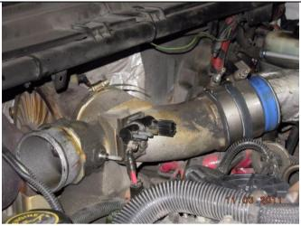
3. Undo the clamps on the hoses from the intake Y to the engine & remove the Y (7/16"), being careful not to damage the o-ring between the turbo outlet & the Y. Put a rag over the air inlets to keep debris out of the engine.
