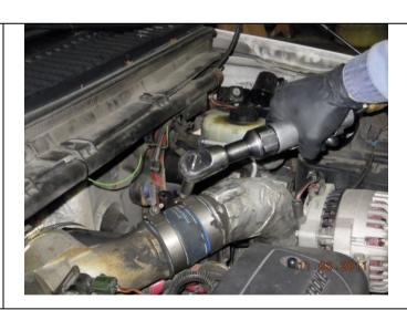
2. Unplug the wastegate controller on the front of the intake Y & disconnect the air intake heater wiring (10mm).
