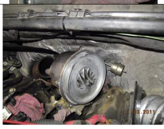
8. Remove the stock compressor wheel (5/8"). Be careful not to bend the turbo shaft. The nut on the turbine end of the shaft is usually irregularly shaped as it is ground down for balancing. A 19 mm or 3/4" T handle socket wrench can be used, if this does not work vice-grips will have to be used.
