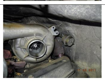
5. Remove downpipe clamp (7/16") & shift downpipe away from turbo as much as possible.
