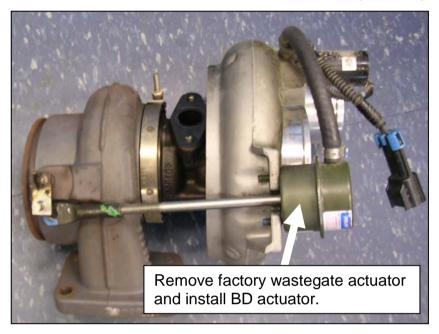
locknut. Apply air pressure to the wastegate diaphram; this should stroke the rod end forward. Align the wastegate arm hole with the BD rod end and insert and lock into place with the supplied cir clip. Once the clip is in place you can then tighten the mounting nuts.
