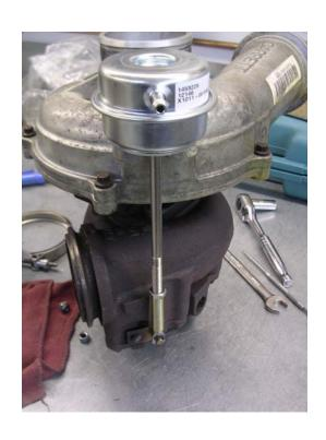
If you would like to adjust the wastegate, loosen the jam nut and slide the rod end off the wastegate lever shaft. Turn the rod end in or out depending on how you want to adjust the boost pressure.
