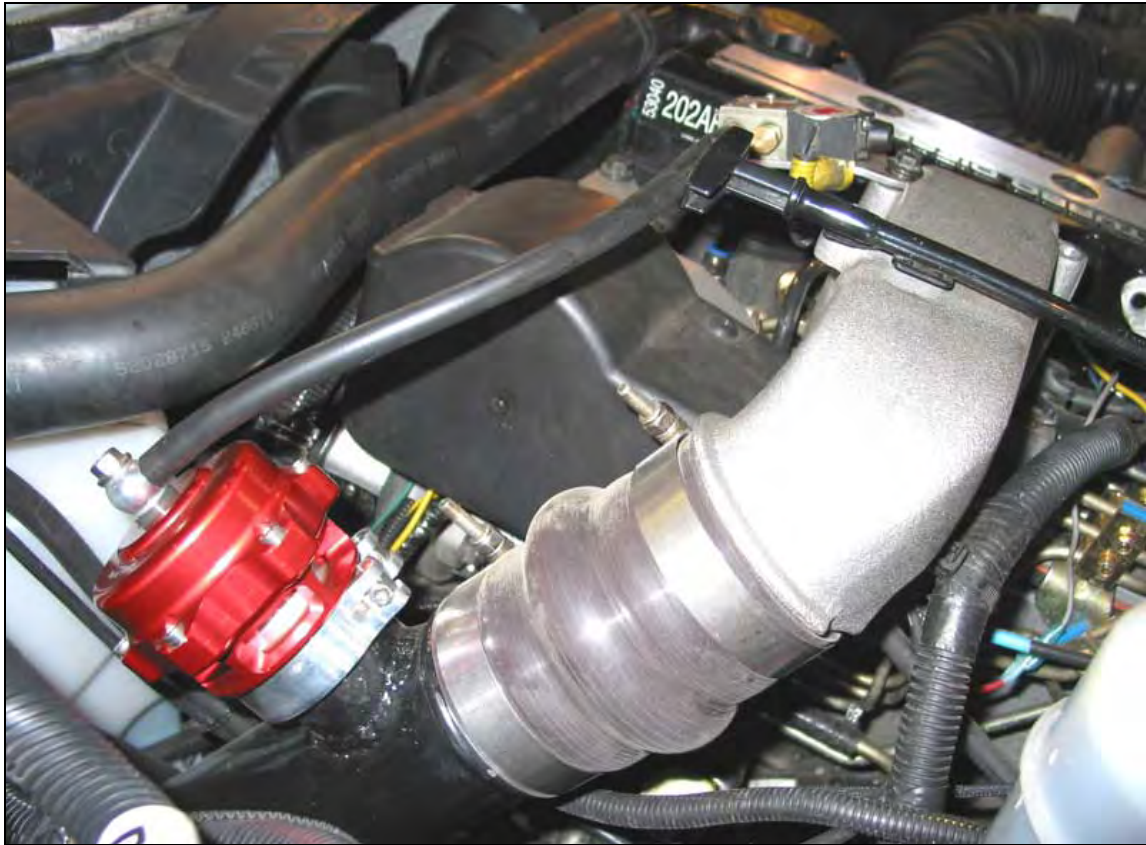
Turbo Blow-off Valve installed in intercooler tube
