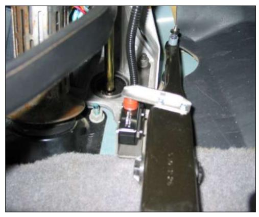
bracket towards the throttle switch on the other bracket you installed above. Ensure sufficient clearance between the long throttle switch bracket and throttle pedal by sliding the bracket as far to the left as possible, to eliminate any possibility of the pedal catching on the bracket.
