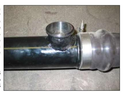
After the weld has been cleaned, a nice coat of black paint is recommended to eliminate any tarnishing.
