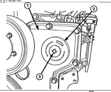
11. Attach C3428B, or L4407 A (or equivalent) gear puller (1) to pump drive gear with two bolts (M8-1.25), and separate gear from pump (a keyway is not used on this particular injection pump). Leave drive gear hanging loose within timing gear housing.
