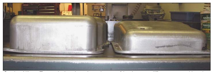
On the Allison Transmission there is a chance of having two different pans. Here is a closer look at both. The smaller one on the right hand side is the most widely used.
