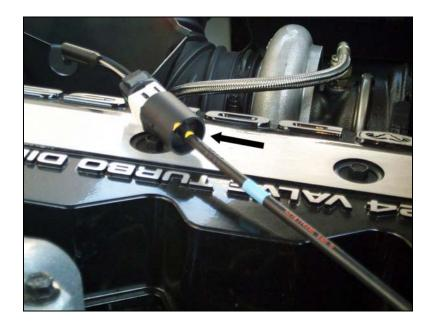
\*\*IMPORTANT: MARK THE CABLE at the original setting before any adjustments are made.
