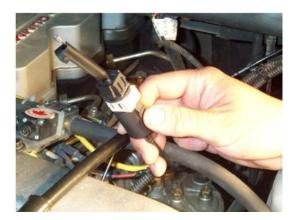
Install white locking clip and then re-install the cable through the support bracket and then on to the throttle lever. Install plastic cover when job is complete.
