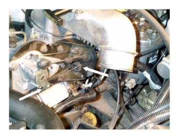
The plastic cover is held in place by 2 plastic Phillips head screws, only light pressure is required to remove them. Do not lose the screws or washers when you remove them. Remove the cable from the throttle linkage and support bracket.
