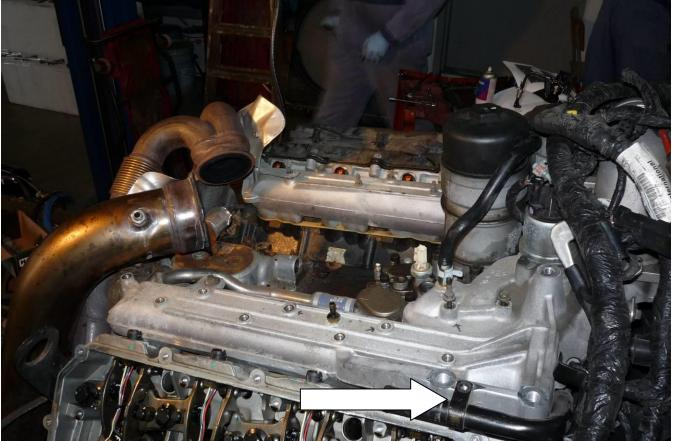
U.S. Shipping Address: 88-446 Harrison St, Sumas, WA 98295 U.S. Mailing Address: P.O. Box 231, Sumas, WA 98295 Phone: 604-853-6096 | Fax: 604-853-8749 | Internet: www.bd-power.com NOTE: Bend back the tab on the rigid metal tube at the RH side of intake manifold to allow manifold to clear.
