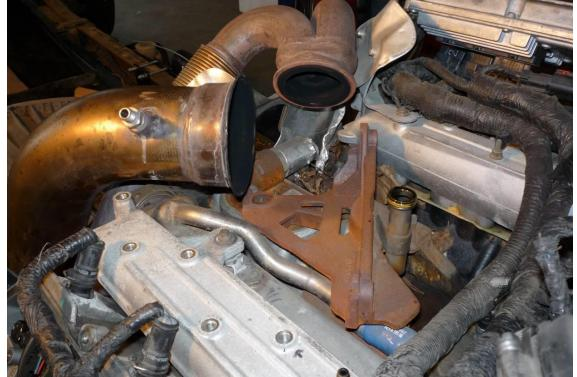
Remove the FICM (Fuel Injection Control Module) by removing two (2) 10mm mounting nuts and two (2) 8mm bolts. Disconnect the three (3) electrical plugs from the wiring harness.
