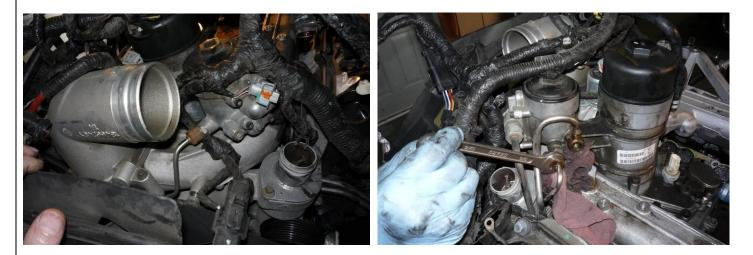
12. Reinstall the oil filter and EGR valve, service both as required.
