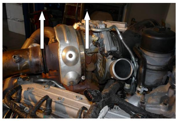
Remove the turbo charger by disconnecting the connector on the turbo solenoid and clip, the oil feed link, exhaust downpipe, and exhaust feed pipe clamp. Remove the three (3) 10mm mounting bolts and pull turbo out.
