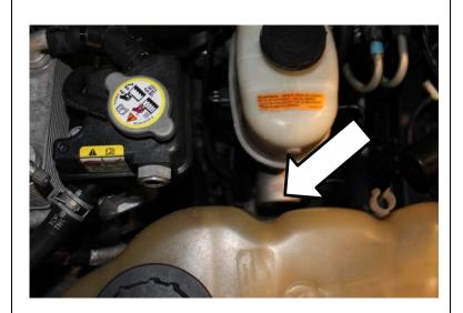
8. Lastly disconnect turbo vane actuator. Connect BD harness to actuator and OE plug.
