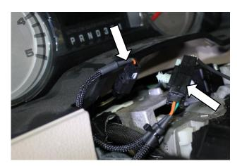
5. Locate the factory purple w/ white tracer wire that connects to the brake pedal switch. Attach the white wire from the BD harness to it using one of the supplied positap. Route harness through firewall (same location as the rotary switch) and connect to module in engine bay.
