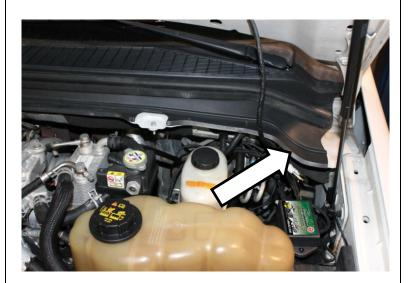
3. Mount switch. Route harness through firewall and connect to module in engine bay.
