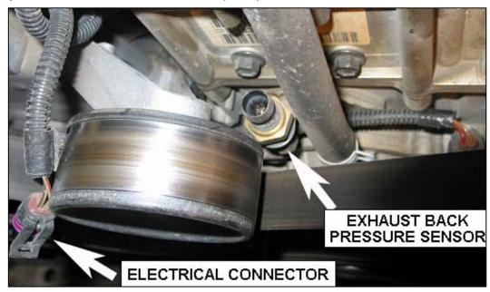
connector. Run the remaining wire away from the belt and the pully and use the nearest engine bolt as a ground.
