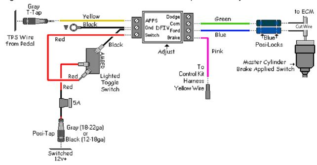
Remove lower section of dash, under the steering column, and mount the DFIV module to the cross member under the steering column. Connect the Black wire from the DFIV module to a good ground.
