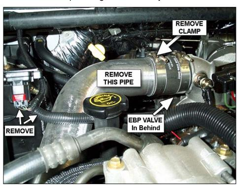
When removing the pipe, the lower rubber bellows that connects to the intercooler rad should remain on the pipe. The pipe slides out of the rubber bellows that is still attached to the intake manifold.
