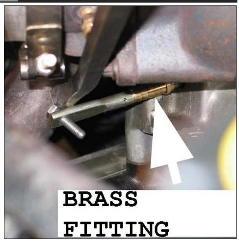
**NOTE**: The clip that holds the rod to the outlet housing is similar to that found on carburetors.
