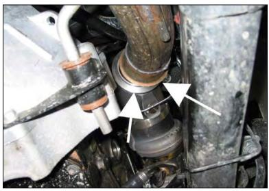
Remove the exhaust elbow.
