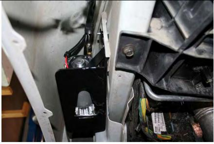
Tighten all bolts to secure the assembly. Route the compressor hose & wiring harness up through the frame opening at the rear of the battery, then route the harness towards the regulator.
