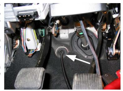
Open the loom and locate the Light Blue w/Black wire and install a gray Posi-Tap™ to it.
