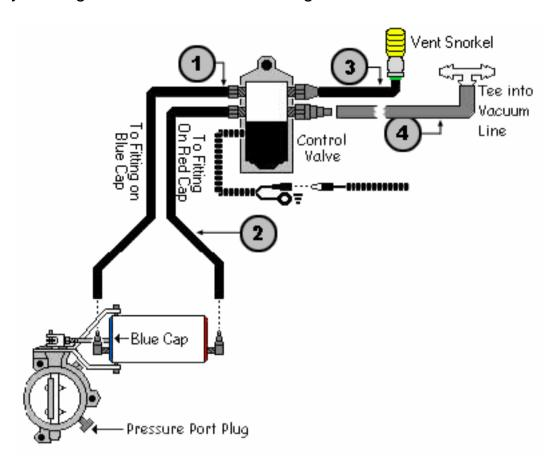
Find the hose running from the vacuum pump to the hydraulic brake booster. Cut this hose just before the vacuum manifold and install the 3/8" plastic tee (w/hose attached) to the two pieces of hose. Attach the free end of the hose (w/plastic tee) to the unused barb fitting on the Control Valve (#4).
