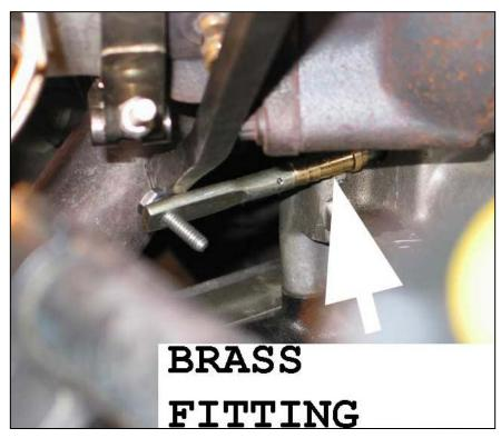
loosen it, then taken out with the use of a swivel socket.
