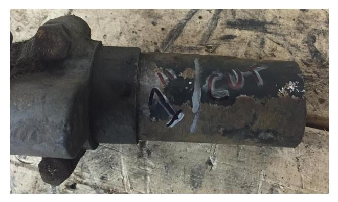
3) Next set the 3/4DD shaft from the kit next to your  $\frac{3}{4}$ " main steering shaft. As shown below, mark that original shaft 3 5/8" above the trimmed shaft for cutoff. The turned down end of the new shaft end will be inserted into the old shaft with a 1/8" gap for welding. The overall length should match the length calculated earlier before this cut off.
