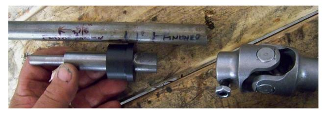
5) For final assembly the lower mast jacket bushing should be secured by either a short sheetmetal screw or pop rivet, being sure that the ¾" shaft will not be bound from free rotation. Then insert the steering shaft through the bushing and add the U joint, positioning it to limit end play of the ¾" steering shaft. If necessary the ¾" washer can be used as a shim. Install the column in the car as you connect to your new steering box or U joint connection to a rack and pinion.
