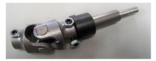
2) Mock up your column to your steering box and determine the length of the complete column including the new U joint. Mark the top of that U joint where it will mate to your ¾" steering shaft. Cut that ¾" shaft ¾" longer to provide ¾" engagement of that joint. Then mark the mast jacket 1" shorter than the ¾" shaft and cut it off square. Deburr the inside of the mast jacket and check the fit of the new plastic lower bushing.
