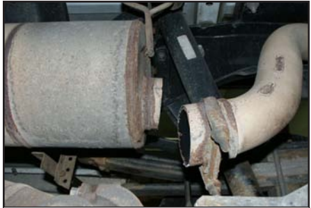
Cut Exhaust directly after muffler
