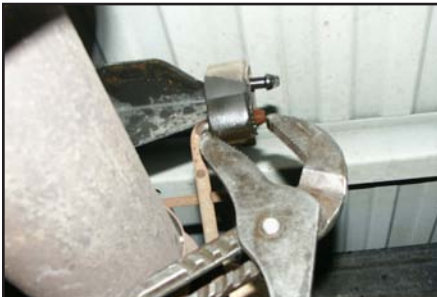
Remove all the necessary exhaust hangers
