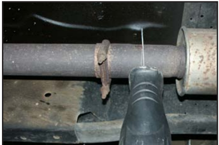
Cut Exhaust in front of resonator
