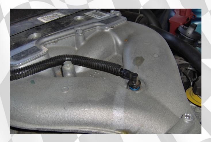
Start with removing the top engine cover and locate the vacuum tube as shown above. This tube runs to the passenger side valve cover where the crankcase vapors are drawn from.
