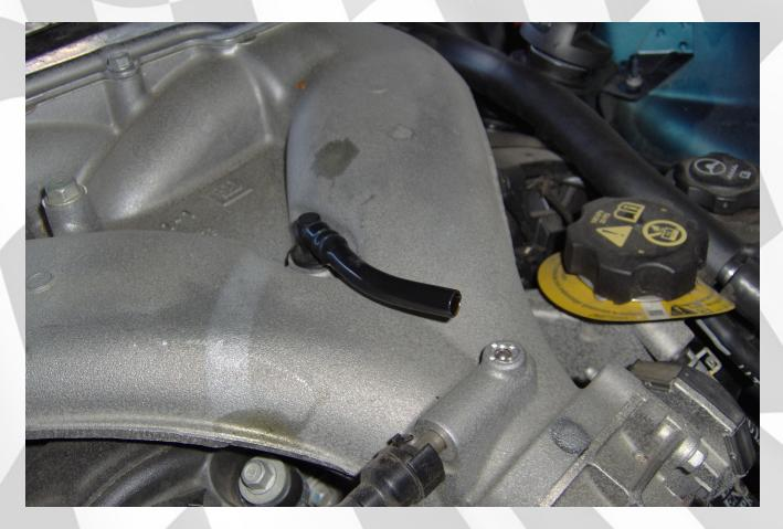
Above shows the vacuum end already cut. It is only oriented in this direction to show where to cut it.
