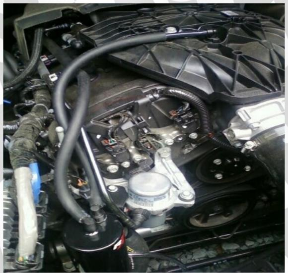
NOTE! The above picture shows the best mount for all makes/models with the LLT or LFX 3.6L engine!!
