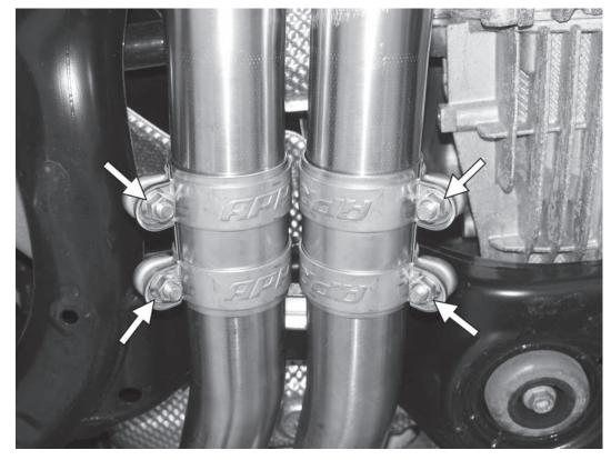
23) Continue the adjusting process on the APR sleeve clamps between the middle section and the rear mufflers. Do not fully tighten the clamps, only snug them up enough where the pipes in them can still be manipulated with enough force.
