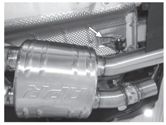
19) Place the right rear APR muffler on the car. Connect the front of the muffler to the right outlet of the APR middle section. Use the factory 13mm bolt to attach the factory hanger back underneath the car. Very loosely tighten the 13mm bolt on the rear hanger.
