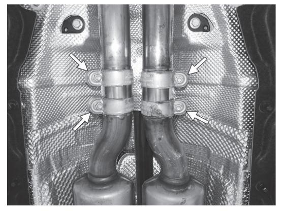
5) Loosen the four 13mm nuts on the stock exhaust clamps at the back of the downpipes.
