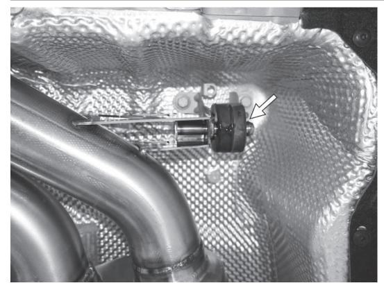
13) Push the hanger from the left side of the APR middle exhaust section into the left rubber hanger that is still attached to the car.
