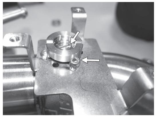
15) On the right rear muffler of the APR exhaust, install the supplied spacer onto the top of the exhaust flap bracket. Ensure the notch on the bottom of the spacer is aligned with the one screw on the mounting bracket that is taller than the other two. Also ensure the rod inside the spacer sits inside the slot at the top of the APR exhaust flap. This slot should also be inline with the exhaust flap inside the pipe.
