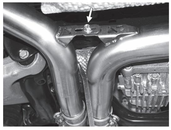
29) Loosen the rear muffler cross brace bolt(s), and then torque the bolt to 25Nm (18 lb-ft). Ensure the position of the rear mufflers do not move while performing this step.
