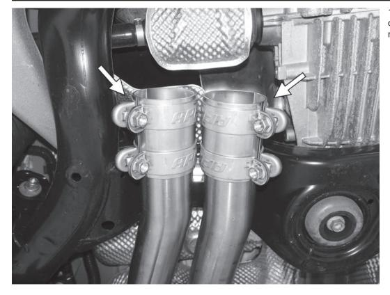
17) Install the two APR sleeve clamps on the back of the APR middle exhaust section as shown.
