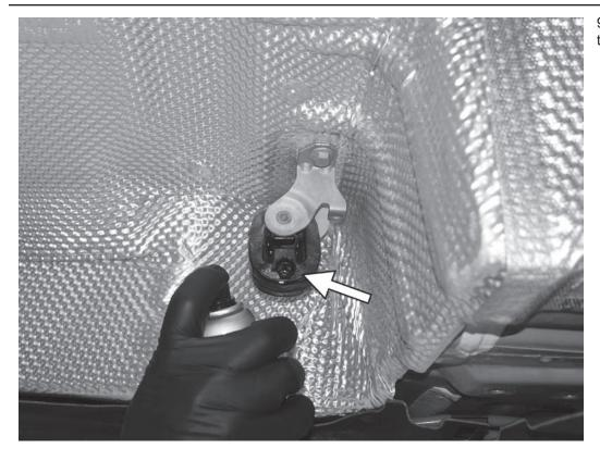
9) Lubricate the two rubber hangers that remain in the middle of the car.
