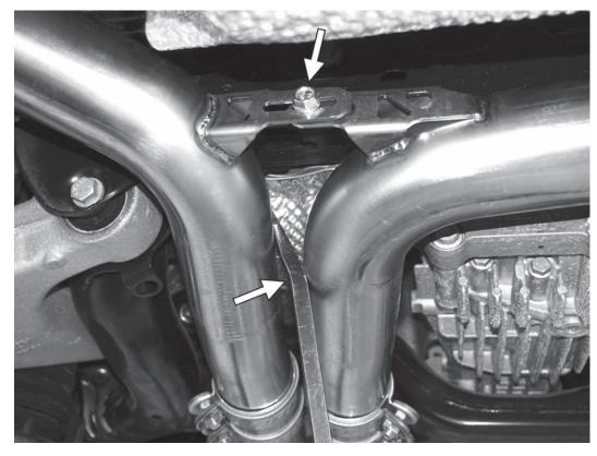
25) Once the rear mufflers are level, adjust the mufflers from side to side so that the outlet pipes are sitting centered in the rear valence. Use a pry bar to separate (or a ratchet strap to bring together) the pipes side to side. In some instances, you will only be able to use one of the two bolts in the cross brace between the rear mufflers. After adjusting the system, tighten down the cross brace bolt(s) and the 13mm bolts on the factory rear muffler hangers.
