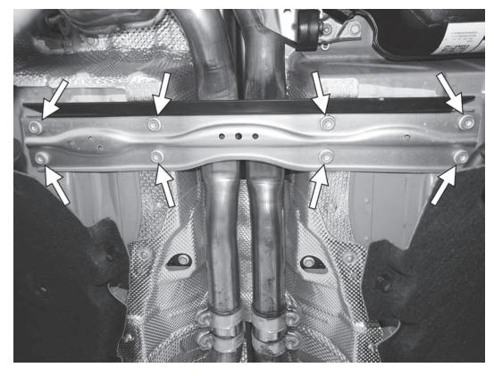
3) Remove the eight 12mm triple square bolts holding the stock cross brace in place, and remove the cross brace from the car.
