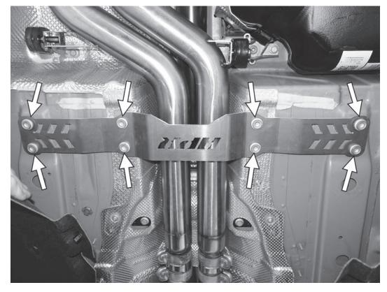
31) Install the APR cross brace as shown with the eight original 12mm triple square screws. Torque all eight to 55Nm (41 lb-ft).
