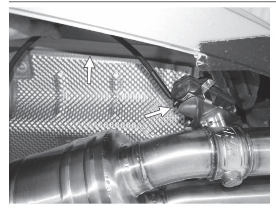
33) Reconnect the factory wiring harnesses to the exhaust flap motors.
