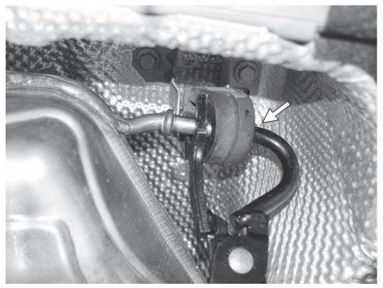
7) With an assistant supporting the rear of the exhaust, separate the stock exhaust from the rubber hangers on both sides in the middle of the car, leaving the rubber hangers in the car.
