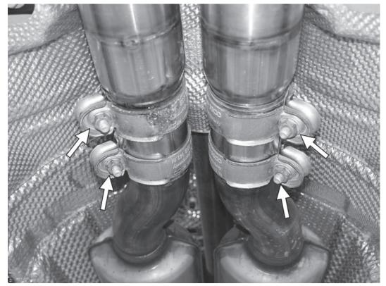
27) Working from front to back, tighten the 13mm sleeve clamps between the downpipes and the APR middle section to 25Nm (18 lb-ft).
