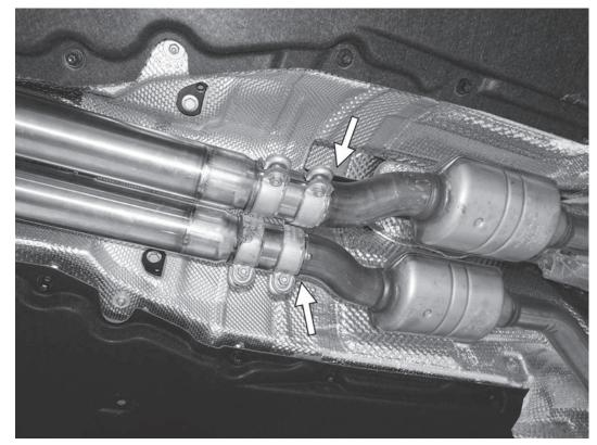
11) Install the middle muffler section to the back of each downpipe. Slide the sleeve clamps in place as shown and very loosely secure them. Ensure the pipes can still rotate inside the clamps for now. There should be approximately a 10mm (3/8") gap between the back of the downpipe and the beginning of the middle exhaust section - do not butt the APR middle section up to the back of the downpipes.
