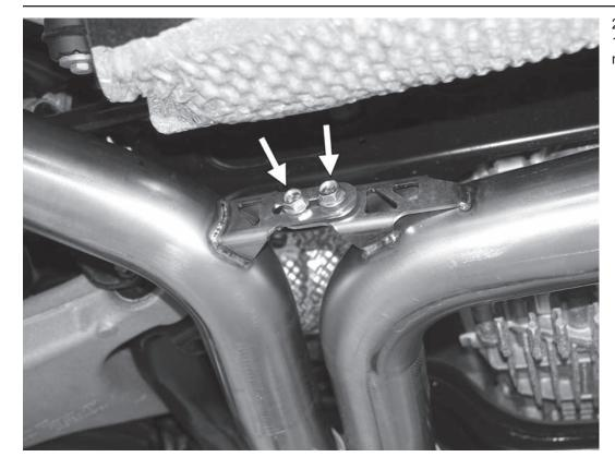
21) Loosely install the two supplied 13mm bolts that hold the left and right rear APR muffler sections together.
